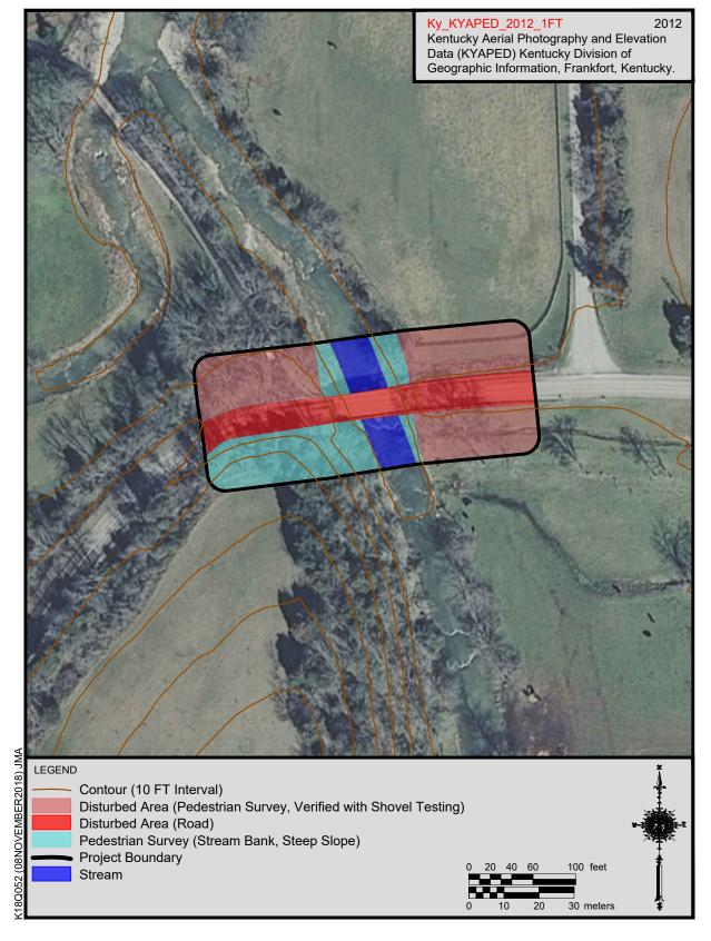
Figure 6. KY 509 bridge over Froman Creek (090B00068N; Item No. 4-1089.00) showing shovel test locations on aerial map.
